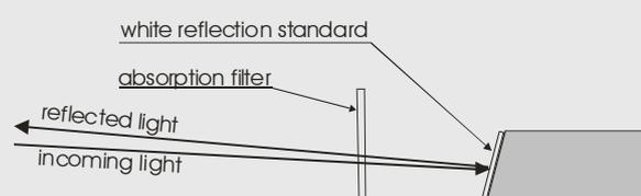
Figure 8: White reflection standard and absorption filter for testing the overall spectral response of a portable instrument.
