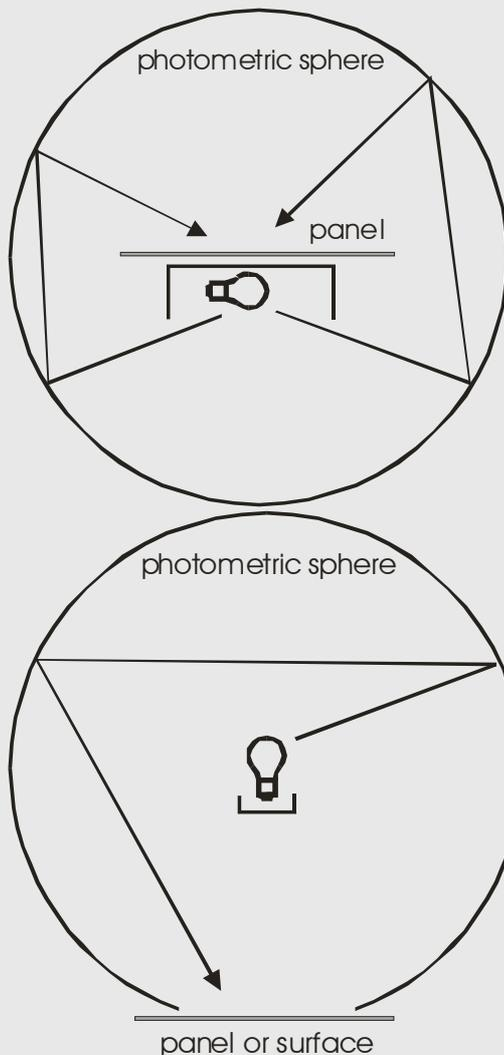
Figure 6: Diffuse illumination by means of photometric spheres.
