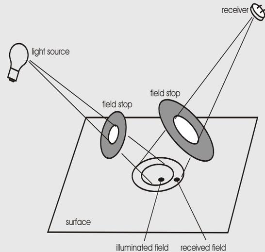
Figure 1: Light source, receiver, field stops and fields.
