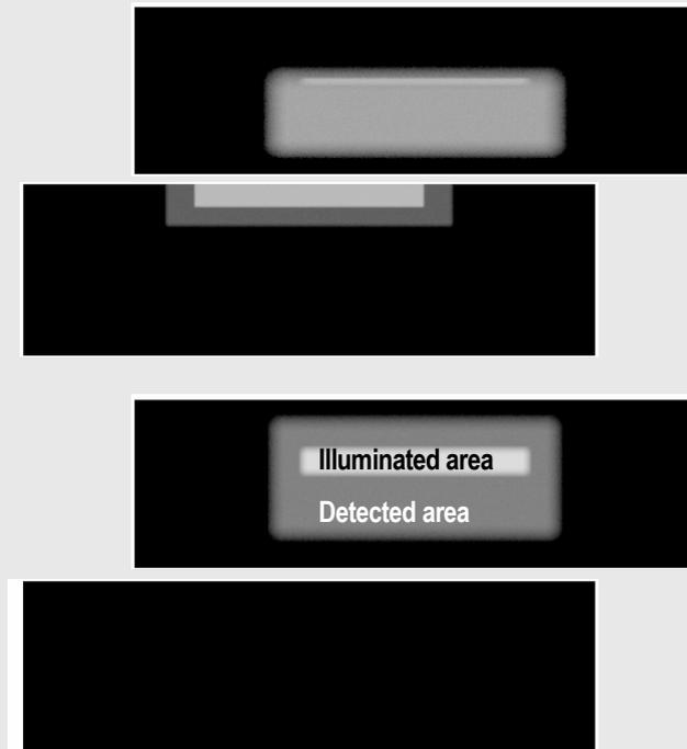
**A:** A critical position, where some light just slips over a profile to fall on the next profile
