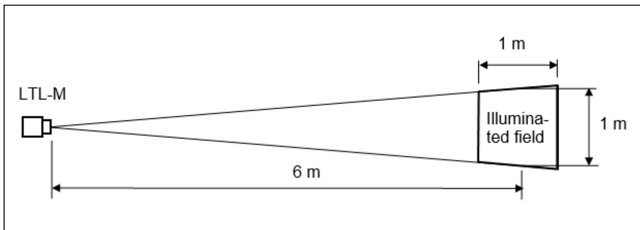
Figure 1: Illuminated field of the LTL-M as seen from above.
