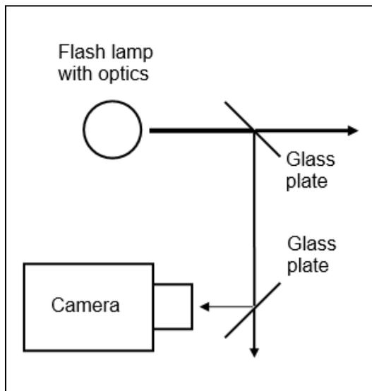
Figure 2: Two glass plates used to give the camera a look to the flashlamp.
