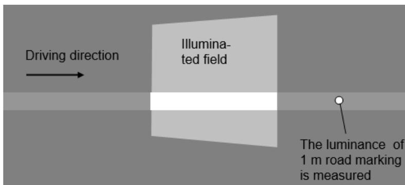
The idea is that, when driving at speed, the illuminated field will be at the location where the daylight luminance is measured in the next image.
