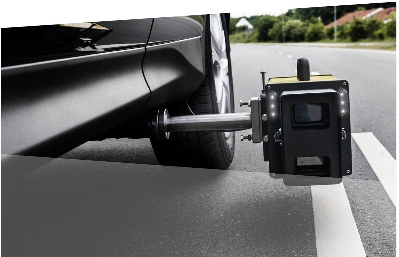
LTL-M is a vehicle mounted instrument for the measurement of the coefficient of retroreflected luminance  $R_L$  of road markings (and road surfaces) in the unit of  $\text{mcd}\cdot\text{m}^{-2}\cdot\text{lx}^{-1}$ . It works by the principles described in section 1.
