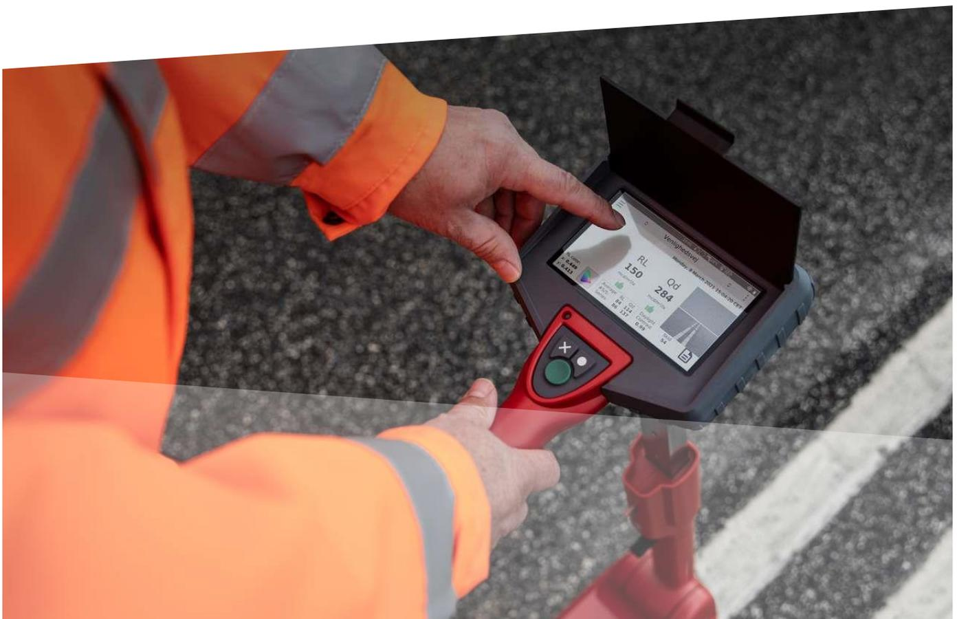
A retroreflectometer is a handheld instrument for the measurement of the coefficient of retroreflected luminance  $R_L$  of road markings (and road surfaces) in the unit of  $\text{mcd}\cdot\text{m}^{-2}\cdot\text{lx}^{-1}$ .
