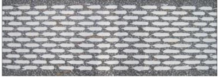
For other profiled road markings, the measured values will vary with the location in the longitudinal direction.
