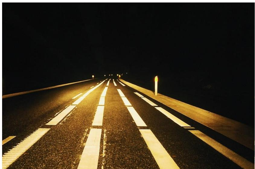
*Figure A.2: Headlamp illumination of road markings – wet conditions.*
