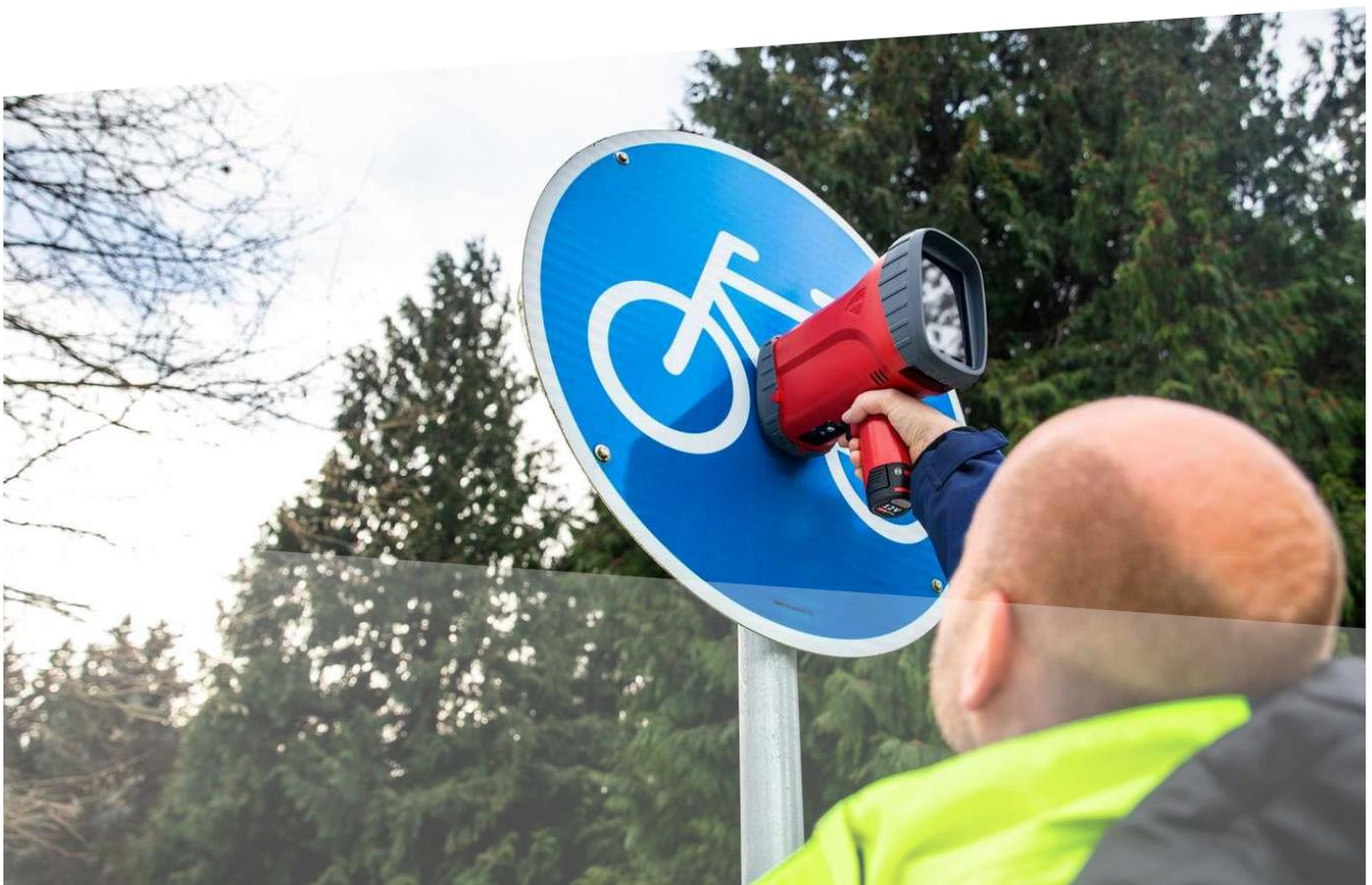
RetroSign GRX is a handheld instrument that measures the retroreflection of surfaces at angular combinations described in standards or regulations for the purpose of testing compliance.
