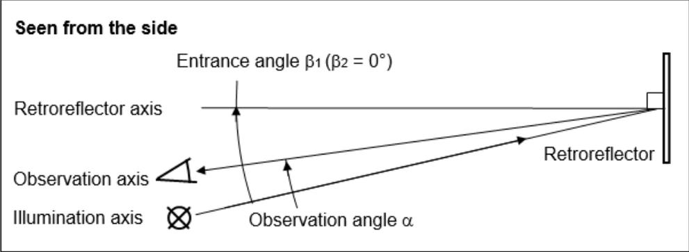
Figure C2: Geometry in two planes.
